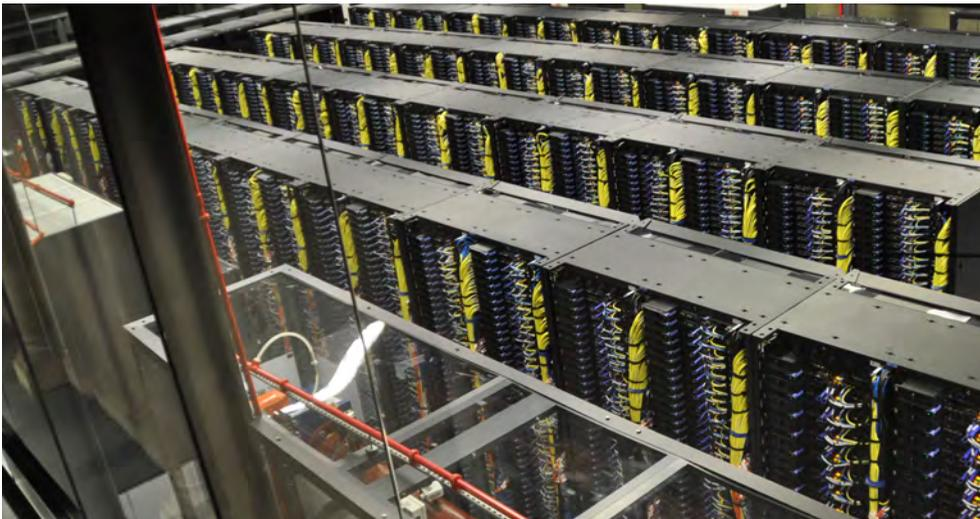
With the upgrade of that year, the MareNostrum supercomputer offered a theoretical maximum performance peak of 1.1 Petaflops (1,100,000,000,000 floating point operations per second<sup>12</sup>). It achieved it with 3,056 servers with
